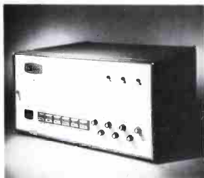
One of time-base correctors to be unveiled is Consolidated Video Systems' new CVS-504, for all non-segmented helical video tape recorders.
