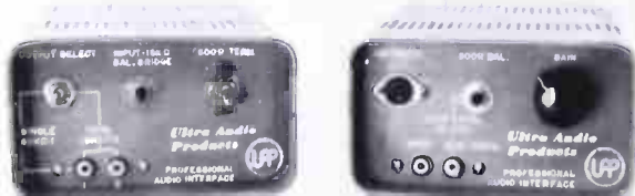
Fig. 3. Audio Interfaces permit proper connection to other sources and leads, overcoming drawbacks of EIAJ VTRs.
