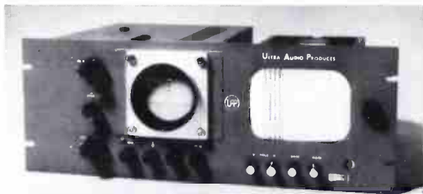
Fig. 2. A waveform monitor (with companion picture monitor, right) gives accurate level indications unobtainable on meters. Low cost units available.
